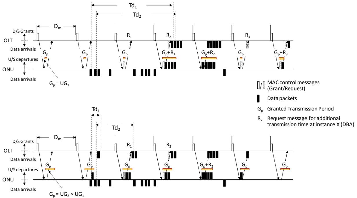
Figure 2 Principle of operation of DBA in a TDMA PON
