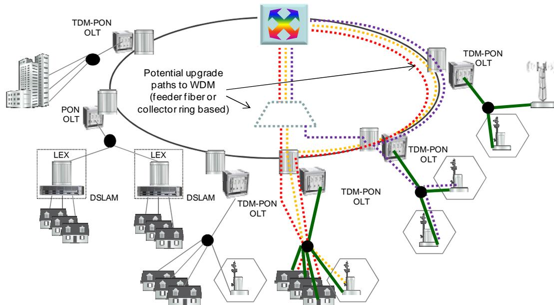
Figure 1: Typical architecture and potential WDM evolution paths (dotted lines)
